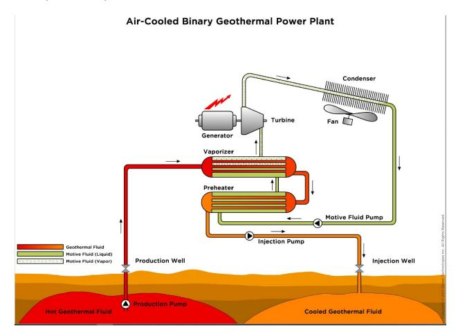
Geothermal fluid leaving the reservoir would be approximately 300 degrees Fahrenheit and would return to the reservoir at a minimum temperature of 150 to 170 degrees Fahrenheit, harvesting approximately 130 degrees of heat/energy. 3-ER-0238 (EA at 2-17).
